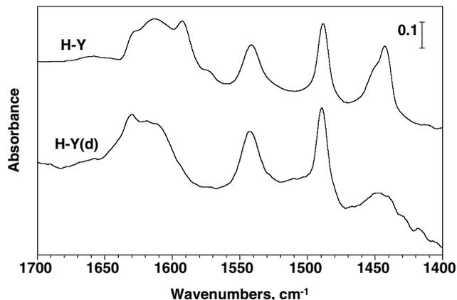
FIG. 1. Difference diffuse-reflectance infrared spectra of chemisorbed pyridine on Y zeolites at 200°C.
