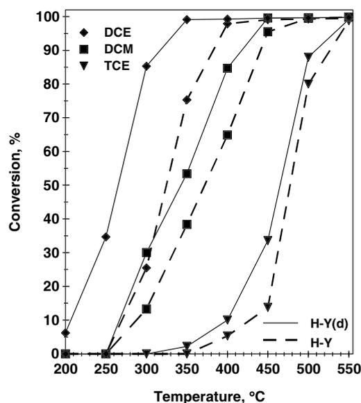
FIG. 3. Conversion of 1,2-dichloroethane (DCE), dichloromethane (DCM), and trichloroethylene (TCE) on Y zeolites vs reaction temperature under dry conditions.
