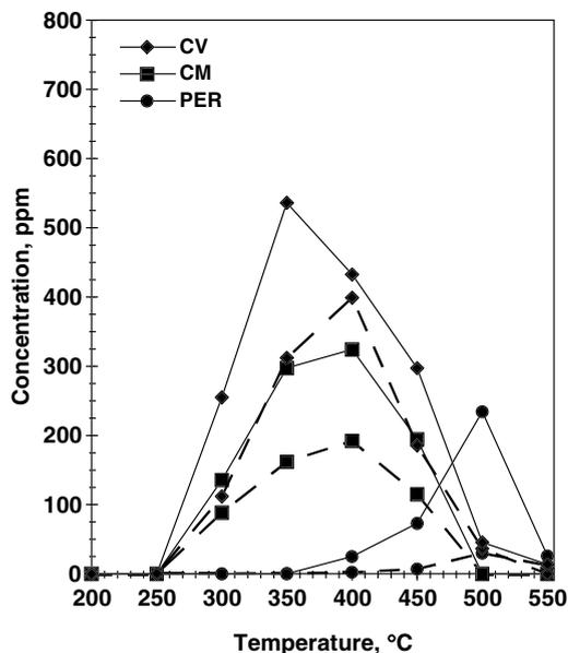
FIG. 5. Concentration profiles of chlorinated intermediates/by-products over H-Y(d) in the absence of water (solid lines) and in the presence of 15,000 H<sub>2</sub>O (dashed lines).
