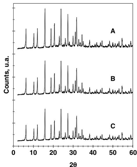
FIG. 6. X-ray diffraction patterns for H-Y(d) zeolite: (A) fresh, (B) after DCM decomposition in the absence of water, and (C) after DCM decomposition in the presence of 15,000 H<sub>2</sub>O.
