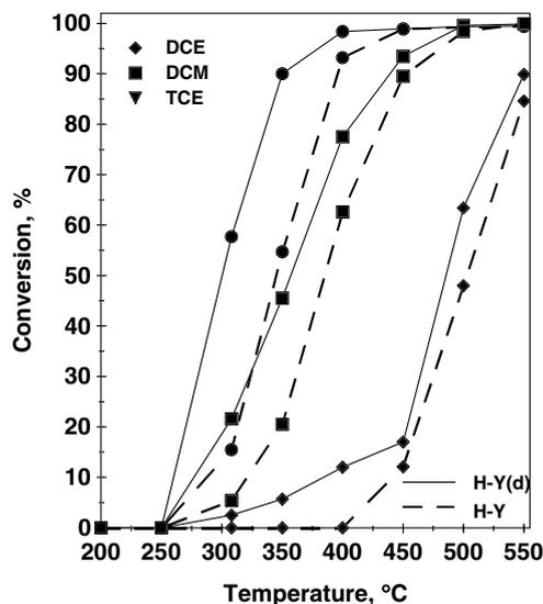
FIG. 4. Conversion of 1,2-dichloroethane (DCE), dichloromethane (DCM), and trichloroethylene (TCE) on Y zeolites vs reaction temperature under humid conditions (15,000 ppm H<sub>2</sub>O).
