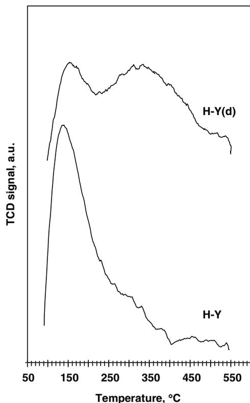
FIG. 2. Acidity of Y zeolites determined by temperature-programmed desorption of ammonia.
